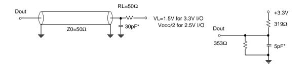
\* Capacitive Load consists of all components of the test environment.
